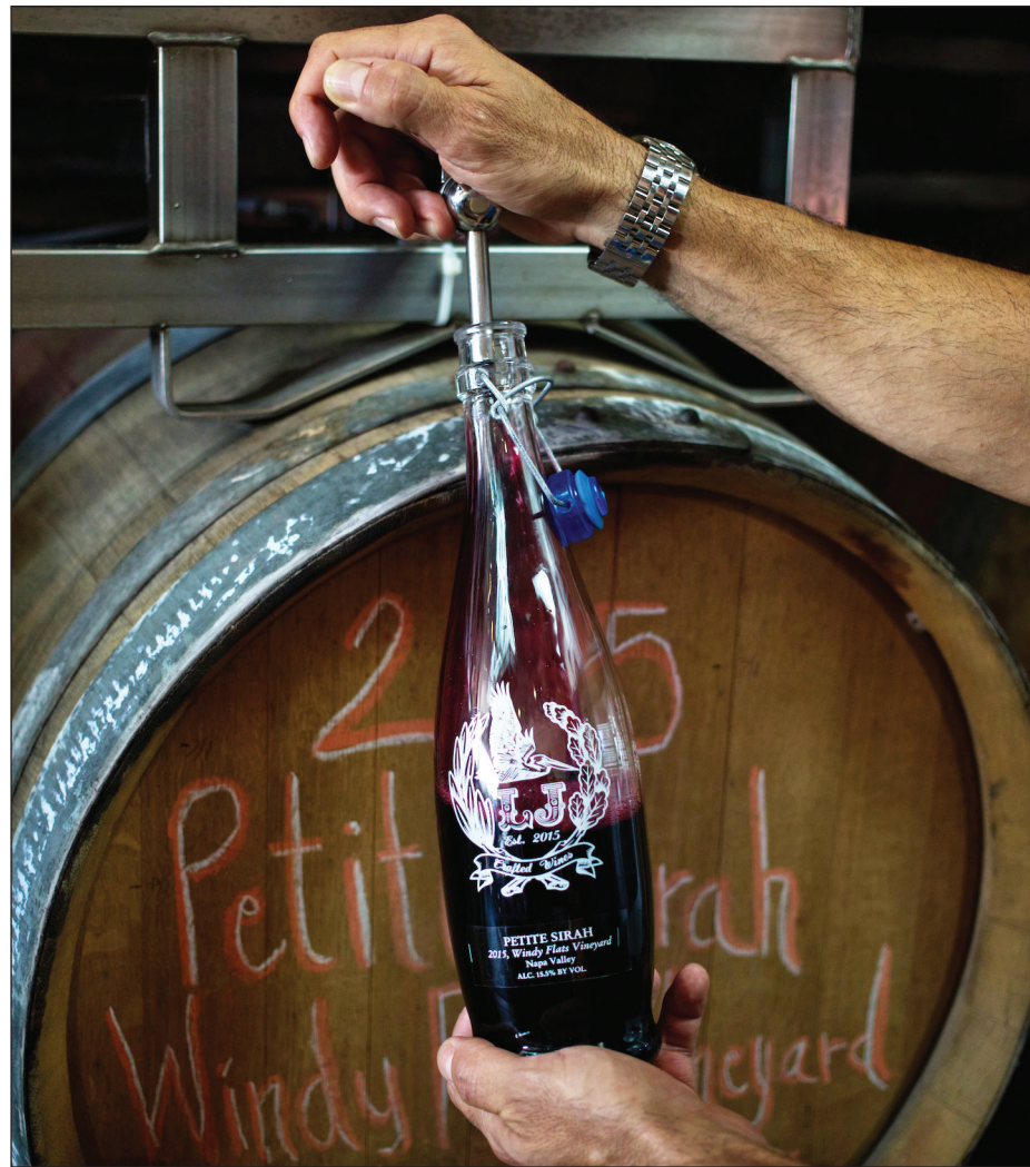
A reusable growler is filled with wine at LJ Crafted Wines using a "wine steward," a device developed by winery owner Lowell Jooste to allow wine to be served directly from barrels without affecting the quality of the remainder of the fermented juice.
